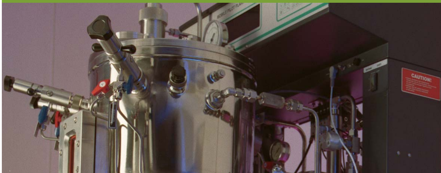
Above 30 liter chemostat—courtesy of Battelle
